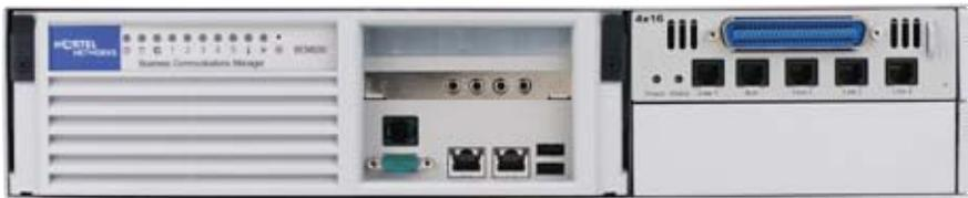
**The compact, all-in-one unit can stand alone on a desktop, be mounted in a standard 19" equipment rack or wall-mounted with an optional mounting bracket.**
